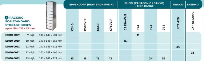
Table shows the maximum number of racks that fit into the model of freezer
