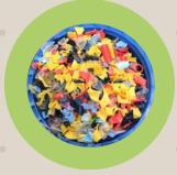
The first step in the recycling process is the crushing of the TipOne® plastic. The shredded material is then processed into plastic granulate
