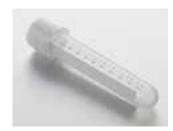
Polypropylene (PP) or polystyrene (PS) sterile tube. White writing area. Graduations marked at 0.25 ml increments. The dual position polyethylene caps can be left loose for aerobic work or sealed for anaerobic culture. Centrifugation rates: 3000 x g (PP), 1400 x g (PS). Temperature use: -190  $^{\circ}$ C to 120  $^{\circ}$ C (PP) / -10  $^{\circ}$ C to 70  $^{\circ}$ C (PS).
