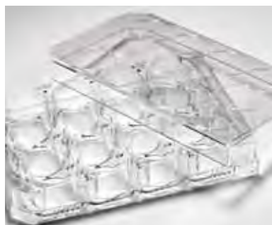
One-way fit lids with condensation rings prevent cross contamination
