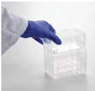
The bottom shells of the refill are nestable to save on waste volume.
