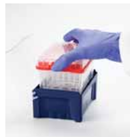
Holding the refill by the finger tabs on either end, place the entire unit inside an empty rack until the wafer clicks into place.
